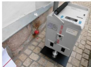
levelling mark to gravity tie
