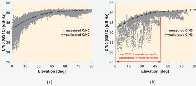
Figure 1: Carrier-to-Noise power density ratio (C/N0) as signal quality indicator, (a) nominal reference curve from laboratory network and 24 hour observation set, (b) observed C/N0 at GRAV12 (Bad Frankenhausen) with the same receiver-antenna combination influenced by urban reflectors.
