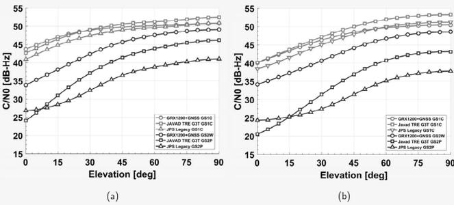
Figure 2: Elevation dependent C/N0 template functions obtained by robot based antenna calibration on a zero baseline approach for several antenna-receiver combinations, (a) Leica AR25.R3 antenna, (b) Trimble Zephyr I Geodetic.
