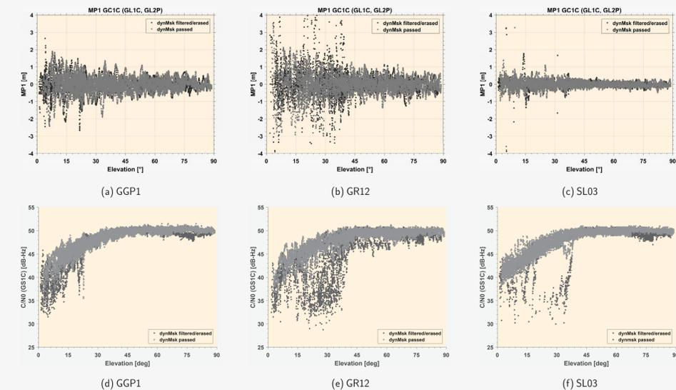
Figure 4: Improvements by applying *dynMsk* on selected baselines on the monitoring network in Bad Frankenhausen, (a-c) multipath linear combinations, (d-f) erased outliers identified by bad C/N0 values (black) provides reduced noise on observations (gray) at low elevations.
