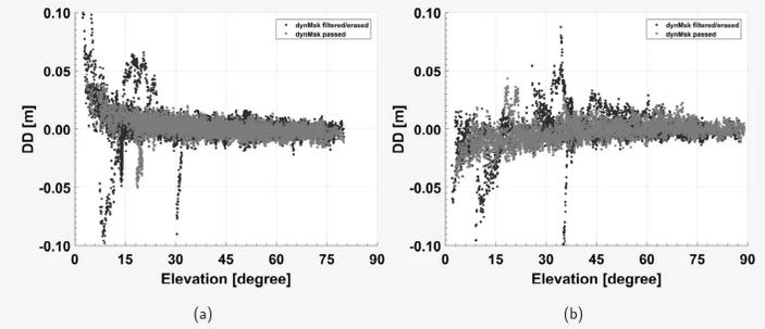
Figure 5: GPS L1 DD OMC for selected baselines in Bad Frankenhausen w/o applying *dynMsk* at both sites, (a) baseline SL03-GGP1, (b) baseline SL03-GR12. Light grey dots show DD OMC obtained by *dynMsk*, black dots show observations, erased by the *dynMsk*.
