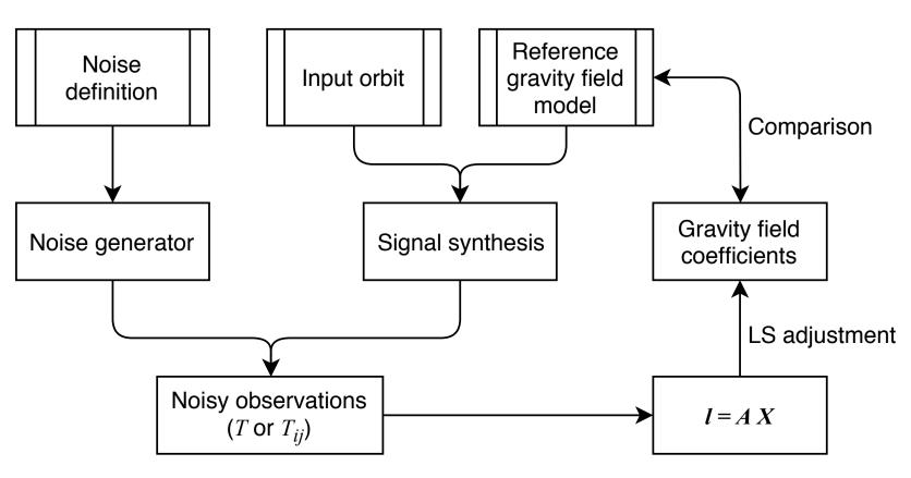
Fig. 3: Scheme of our closed-loop simulator for gravity field recovery from clock and CAI data. The observation signals are synthesized from a background model, e.g., EIGEN-6c4. The noise is generated based on the specifications of the sensor behavior. A rigorous Least-Squares (LS) adjustment is applied to retrieve the gravity field coefficients, which are compared to the input model for evaluation.
